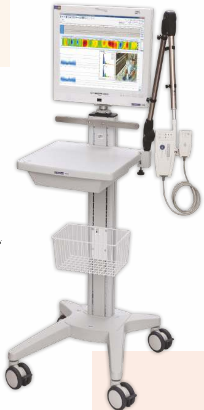
3-channel EEGDigiTrack CFM unit installed on the medical computer and medical cart
